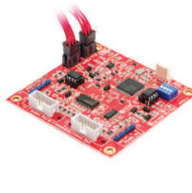
INTG-996520PCB&K Integrati UniBus 2 Port RS-232/RS-485 UART PCB & Accessories (Includes 270mm UniBus patch cable)
